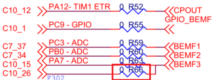
Figure 4-6. X-NUCLEO-IHM07M1 Board Circuits Modification for NUCLEO-F303RE
