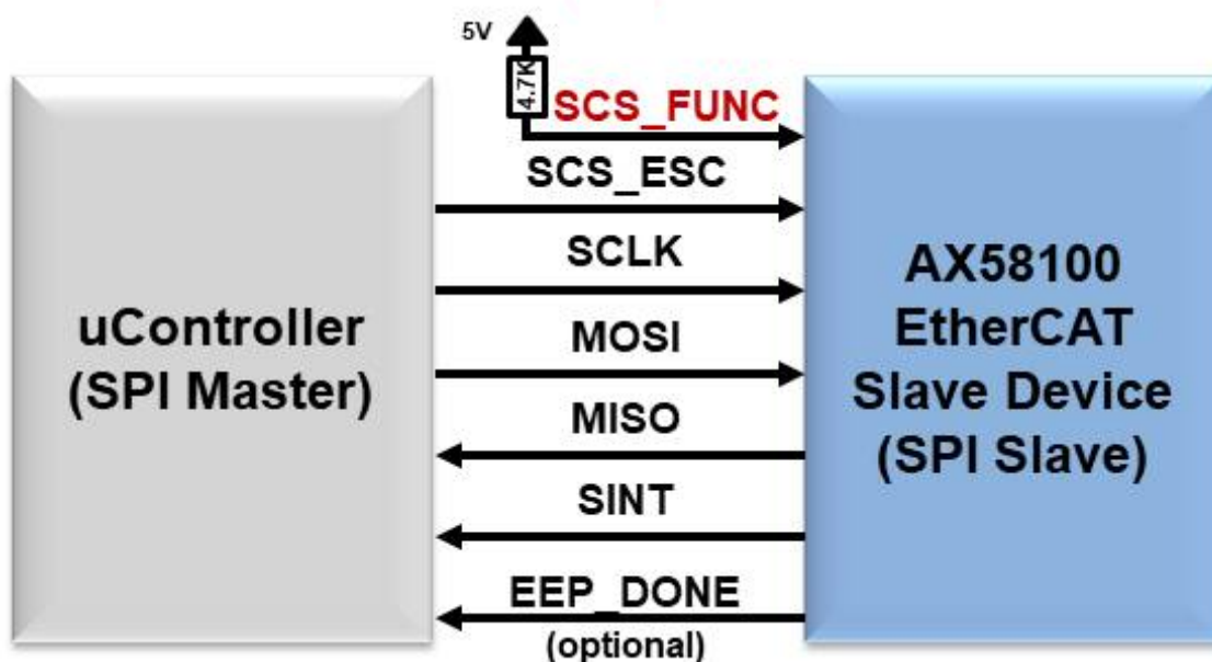
Figure 2-3. AX58100 ESC PDI SPI Slave Interface Connection
